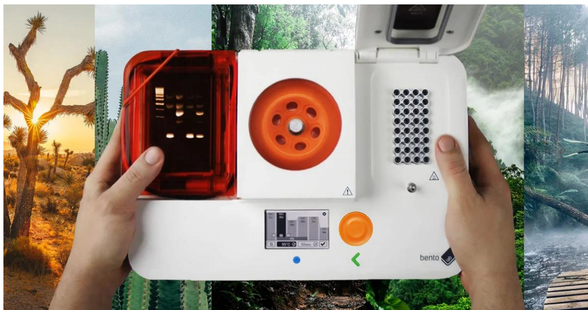
Fig. 1. Portable Bento lab for DNA extraction, amplification and gel visualisation. Photograph © Bento Bioworks Ltd 2024.
